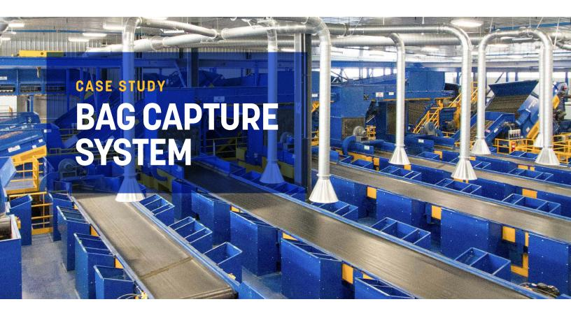
Rumpke Waste and Recycling provides curbside waste collection services and operates landfills and recycling centers across Ohio. AES was selected to provide a plastic bag capture system for their new \$32 million MRF in Cincinnati. Plastic bags in the waste stream reduce the value of recyclables, clog process machinery and pose a danger to workers tasked with removing tangled bags from the equipment.
